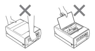
• When putting the printer down, put the back feet of the printer first, and then put the front feet down slowly.
